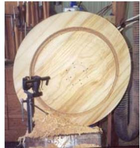
Gordon has a small crane to load the big blanks on the lathe and it took some persuasion with the grinder to get the blank to clear. He used a coring tool to remove the center sections.
