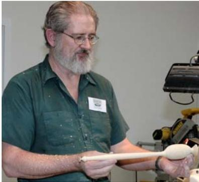
Once the sanding on the handle is complete then the blank comes off the lathe. The ends are trimmed on the band saw then the inside of the spoon bowl is cleaned out with a power carving tool. This results in a spoon bowl that can be oval shaped to match the profile that was turned in the first step. Tony also demonstrated his fixture for turning the
