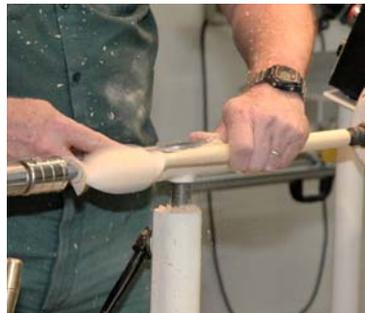
Now the spoon handle is formed while the spoon bowl is offset. For all of the turning, Tony only used spindle gouges. He did follow Alan Lacer's example and used a dead center on the drive end to allow for slipping during a catch. The
