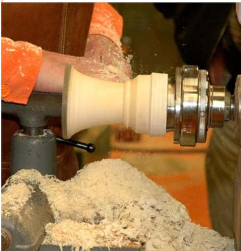
Ken will sand to the final sanding then use various drying techniques with newspaper and paper bags to slow down the loss of moisture and potential cracking problems. Thanks Ken for a great demo.
