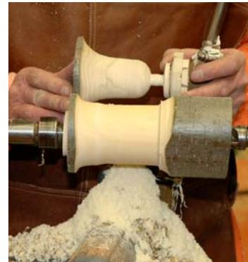
First the wet branch is turned between centers to establish the basic shape and to make a foot to allow for chucking to the bottom.
