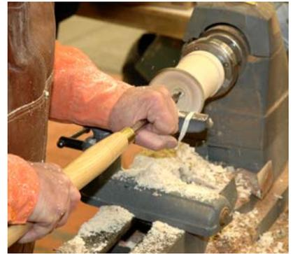
Ken's tool of choice for hollowing the inside is a ring tool. There was some debate if it is better to hollow out the inside first or to hollow after the outside shape has been turned. Ken's preferred method is to hollow the center then cut the outside to follow the curve.
