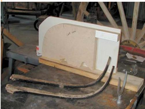
Harlan is making new dash support pieces for a sleigh he is rebuilding. The pieces to the left need to be replaced because the tenons are rotted away. Harlan will also show past steam bending project results.
