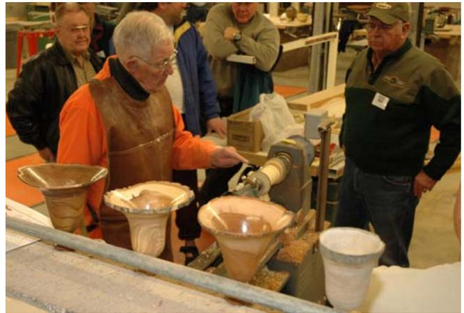
The vase is then chucked by the foot end to allow access to the top end so it can get hollowed out. The first weapon is a gouge to true up the end. The bark is left on the top end.
