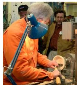
for discussion and for Ken to sharpen his tools. He did all of his sharpening on the grinder without a jig. As Ken worked the bowl inside progressively deeper he showed the body movements that were necessary to get the correct tool angle to get a good cut. Sometimes Ken will work from the
