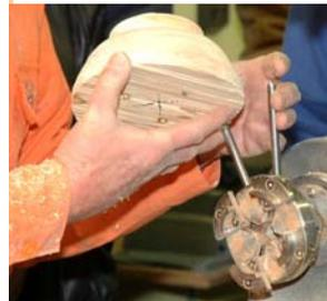
Ken attacked the inside of the bowl to remove the material. The same bowl gouge that Ken used on the outside of the bowl is also used to remove the material from the inside of the bowl. The cuts are repeated until the desired bowl thickness is achieved. A few stops in the action were necessary
