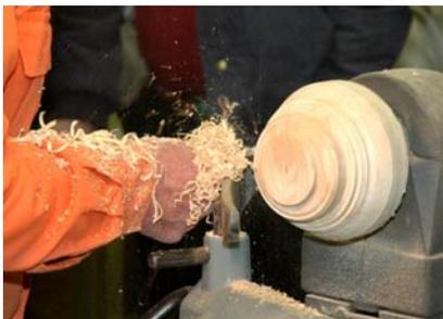
turned a foot or spigot on the bottom of the form to allow gripping by a chuck. After removing the form from the face plate it is turned around and gripped on the bottom by the chuck to allow turning of the inside of the bowl. Some shaping on the outside can still be done but it is best to have the outside cuts mostly done while the bowl is on the face plate. Once the bowl form is in the chuck then
