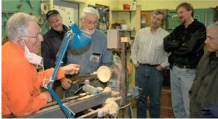
Gordon stepped in also to demonstrate a technique he described as a 'Shear Scrape'. This allow further refinement of the outside of the bowl after it has been reversed onto the chuck. Everyone enjoyed the demo. At the end Ken was unsure if he would finish the bowl or if it really would end up on the firewood pile as originally promised.
