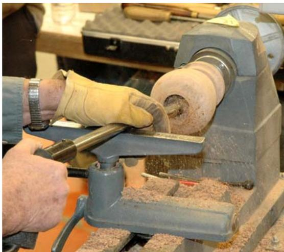
This is a very difficult surface to sand so it is necessary to clean it up with a scraper.
