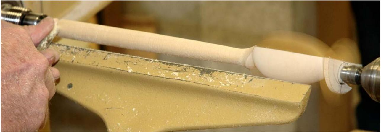
Remove the blank from the lathe and trim off the waste ends, blend in and finish sand the ends.
