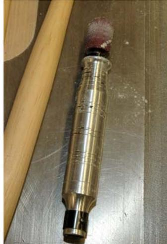
To hollow out the bowl of the spoon, select a method that is available to you such as: a power rotary carver i.e. Foredom or Dremel, or use carving gouges. Then sand off the remaining paper on the rim of the spoon bowl with a sanding block to keep the bowl flat.
