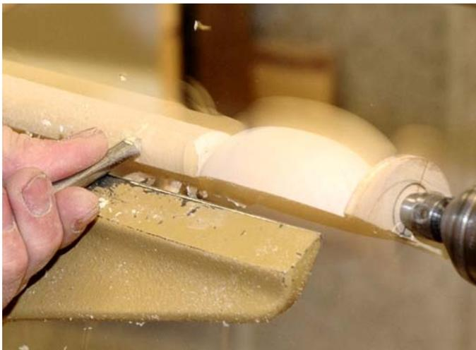
Shape the handle however you would like (the possibilities are endless), and sand the handle. At this point you may turn into the waste areas as much as you are comfortable with.
