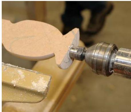
Mount one of these blanks between the cup centers on the centerline of the desired handle, the spoon bowl will be off-center. Use marks #3 on both ends.
